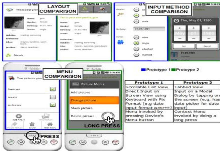
Figure.3 BDroid prototypes and feature comparison [1]
